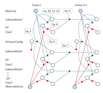
Fig. 4. Factor graph [18] representing the proposed CRF model for articulatory feature forced transcription. The shaded nodes represent variables that we condition on. The red and blue square nodes represent factors, each of which is a non-negative function defined over the configuration of the set of variables connected to it. The number in the dashed box corresponds to the equation(s) in the text that implements the corresponding factor.
