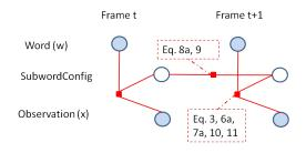
Fig. 5. Factor graph representation of final simplified model after sub-word state variables have been collapsed to obtain a linear chain. The numbers in each dashed box correspond to the equations in the text that implement the corresponding factor.
