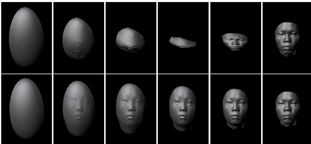
Figure 8: Interpolating an ellipse and a face. Top row: Method of Section 3 without manual interaction. Bottom row: Results of the automatic interpolation method described in Section 4.
