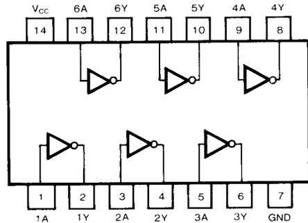
Suffix-Blank: Plastic Dual In Line Package
