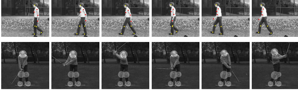
Fig. 10. 2D Tracking using the WSL tracker. Top row: Tracking the chest, knees, head, ankles and visible arm. The tracked upper body joints are shown in red, with the head and tracked lower joint points shown in yellow. Bottom row: Regions used for tracking the ankles, knees, and head are shown.
