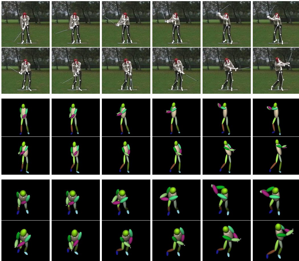
Fig. 14. Monocular Tracking a full swing in a 45 frame sequence. First two rows: The skeleton of the recovered 3-D model is projected into a representative subset of images. Middle two rows: Volumetric primitives of the recovered 3-D model projected into the same views. Bottom two rows: Volumetric primitives of the 3-D model as seen from above.
