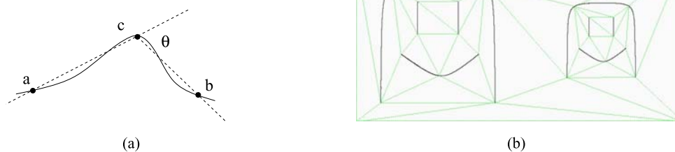
Fig. 6 Building a discrete graph structure from bottom-up. (a) We take a contour detected by a local edge operator Pb and recursively split it until the angle \theta (a scale-invariant quantity) is below a threshold. (b) We complete this piecewise linear structure with constrained Delaunay triangulation . G -edges (gradient edges detected by Pb ) are in
