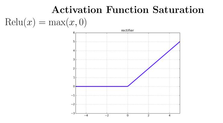
The Relu does not saturate at positive inputs (good) but is completely saturated at negative inputs (bad). Alternate variations of Relu still have small gradients at negative inputs.
