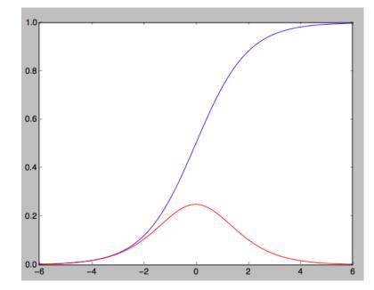
The gradient of this function is quite small for |x| > 4. In deep networks backpropagation can go through many sigmoids and the gradient can "vanish"
