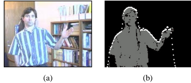
Figure 3. (a) Input. (b) Draped segmentation. The dots represent point masses, connected to their neighbors by springs.
