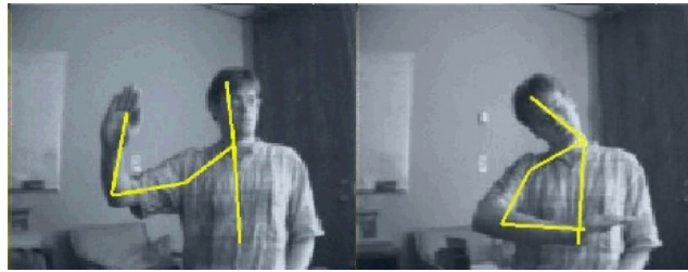
Figure 7: Two frames demonstrating the initialization and tracking in the presence of self-occlusions. One set of lines connect the neck, shoulder and elbow joints, while the line segments on the lower arm, head and torso extend from the joints in the direction of the appropriate blob centers but go further so that their lengths represent the sizes of the blobs.
